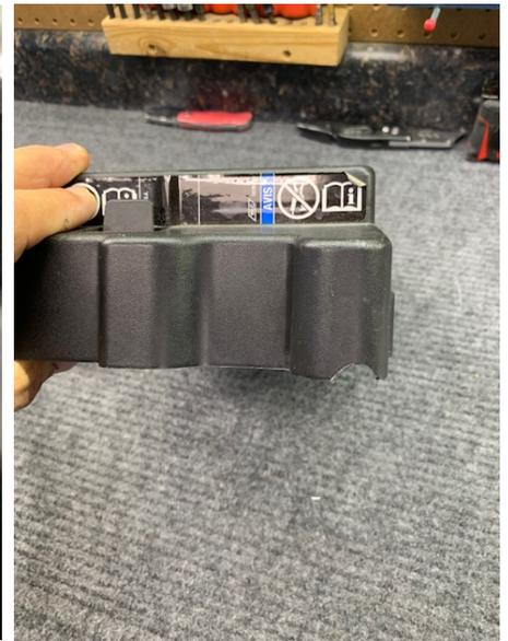
11. You will need to slightly modify the Fuse Box cover by putting a small rounded notch on the corner to clear the fan wire. It should look like the right photo above. Check the fit....
