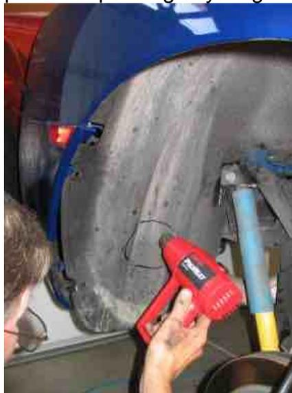
22. Once you are satisfied with your “molding” around the corner of the battery box and that there is no stress on the fascia tabs, reinstall the two fasteners to the rear fascia. You will have a lump showing in the fender liner where the corner of the battery box is in contact. This is normal and to be expected. You will not have any clearance issues with the tire.
