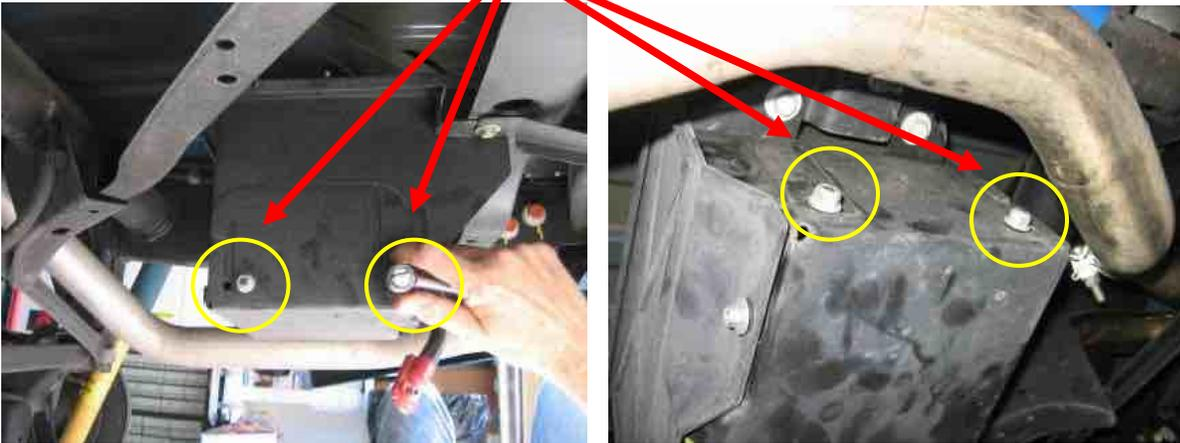
7. Drop the battery box into the lowered position and remove the hold down. The battery (about 40lbs!!) can now be .....carefully removed from the carrier.
