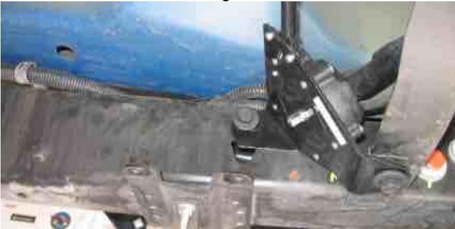
14. Install the new ground cable to the studs on the frame and body. I let the cable lay across the top of the shock absorber as shown in the left photo and then routed the positive cable above it as shown in the right photo. This will look and lay different with the fender liner still in place, but you'll figure it out. The positive cable must be above the ground cables.
