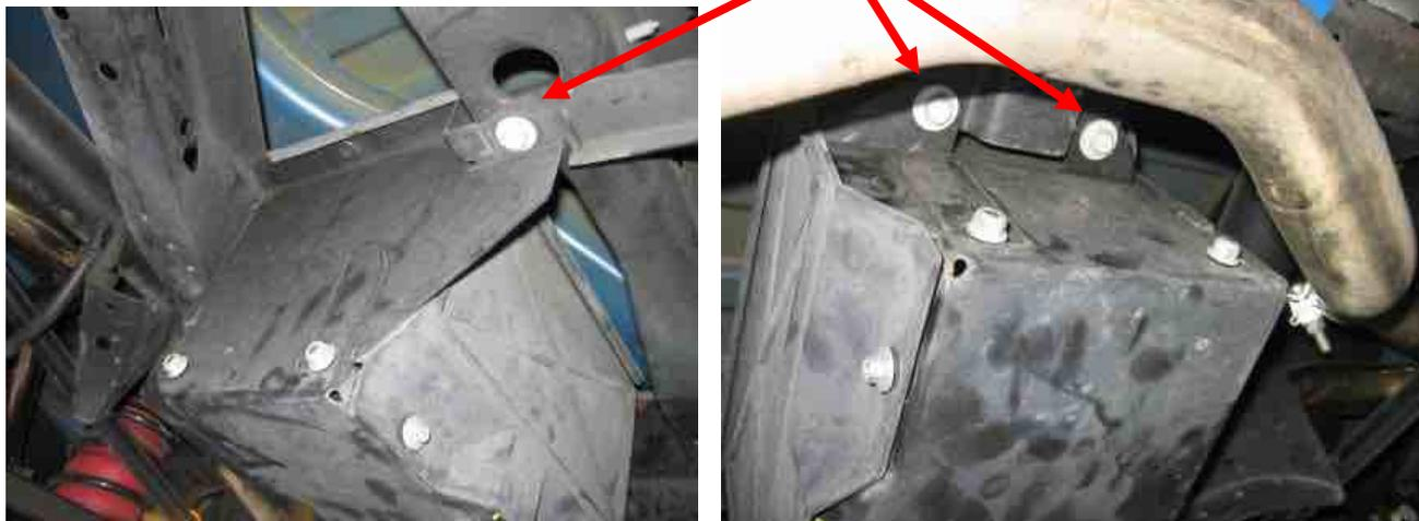
9. Remove the angled rear fascia brace (the one that was held in place by one of the battery box bolts) that is bolted to the back side of the license plate area. Install the aluminum brace that is in the kit and bolt it securely in place. Note that the aluminum is 6061 and will hold its shape, even after you “tweak” it a little to make it fit just right.
