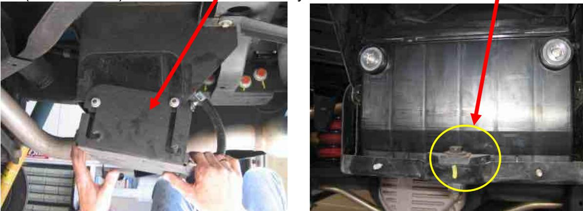
8. Remove the 4 bolts that hold the battery box in place and remove the box from the truck.
