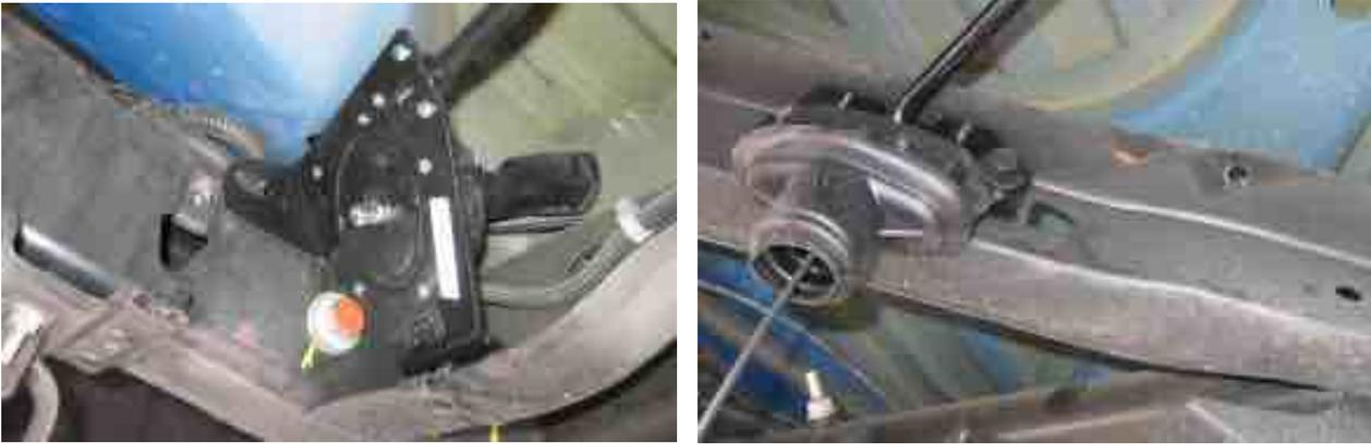
13. Pull the hoist out of the corner, get it positioned over the nut plates and install the two 10mm bolts. You can now tighten all three of the hoist bolts.
