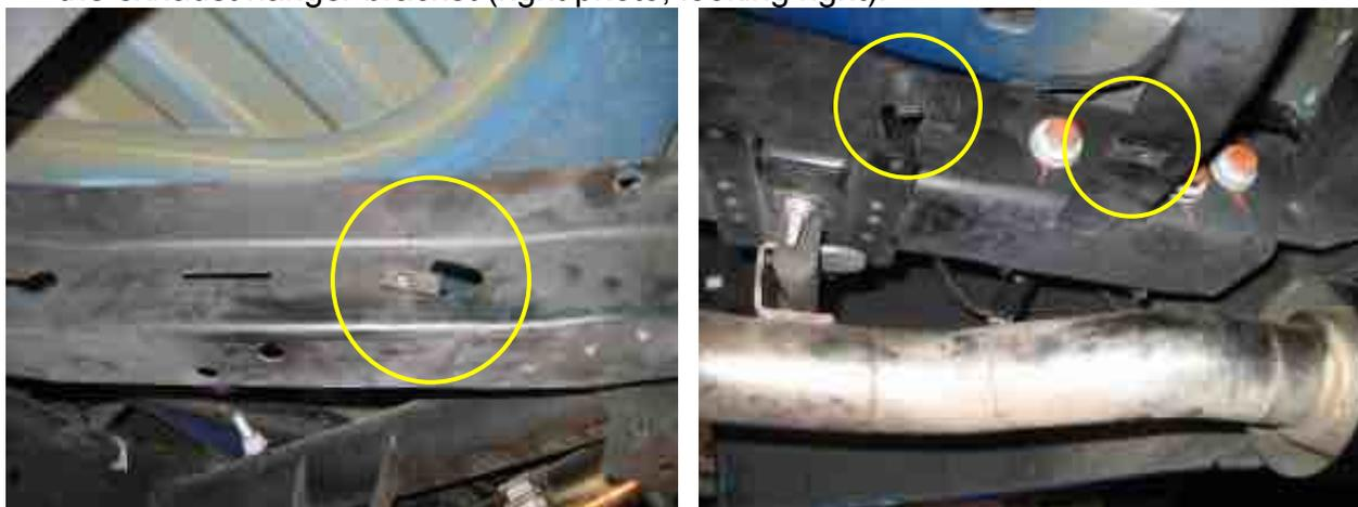
12. Put the GM tire hoist as far into the corner of the SSR as possible (left photo), so that you can get the mounting tab into the slot in the diagonal crossmember. Patience and perseverance is key here. If you get it positioned just right, the hoist will slip into the slot perfectly and you can install the bolt (right photo)... Don't tighten it yet.
