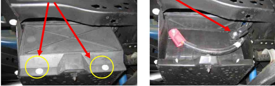
6. Loosen the 4 battery box nuts so you can drop the battery into the lowered position.
