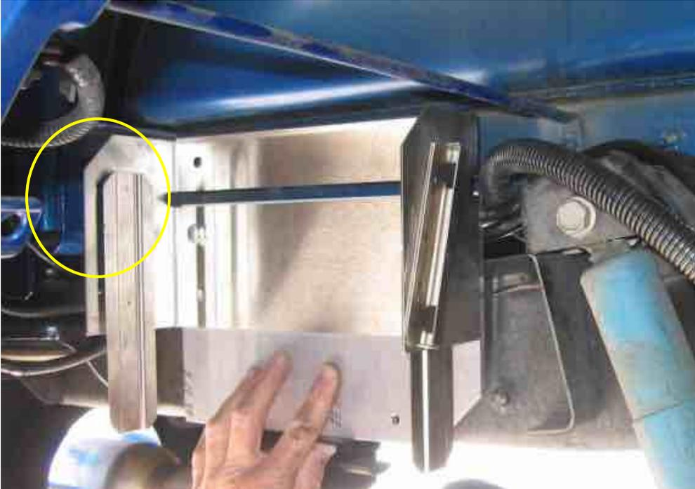
17. Clamp the bracket assembly to the frame of the truck and install the 4 stainless Tek screws into the frame with an electric drill and the 3/8" hex driver.
