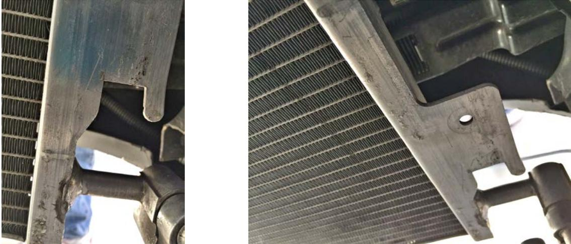
Lower Passenger side condenser bracket after modification
