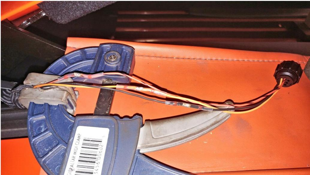
12. Stretch the original protective wire sleeve up to the new connector and secure it in place with the piece of adhesive-lined heat shrink tubing that you have on the wire sleeve. The shrink tubing will lock into the threads on the connector and glue itself to the sleeving.
