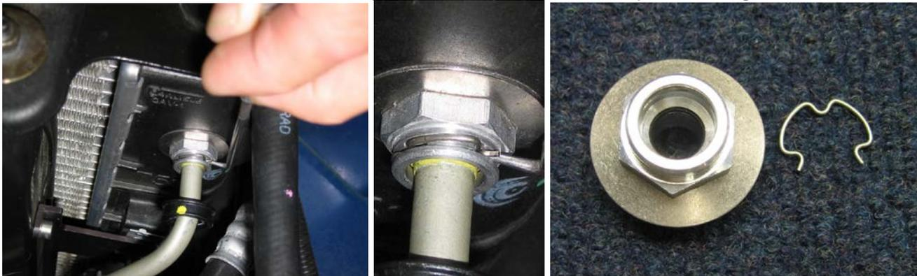
7. Using your hands, carefully twist the upper fluid line about 30 degrees toward the right side of the truck. It should be pointed to miss the radiator tank and will have the end actually parallel with the air conditioning hose.
