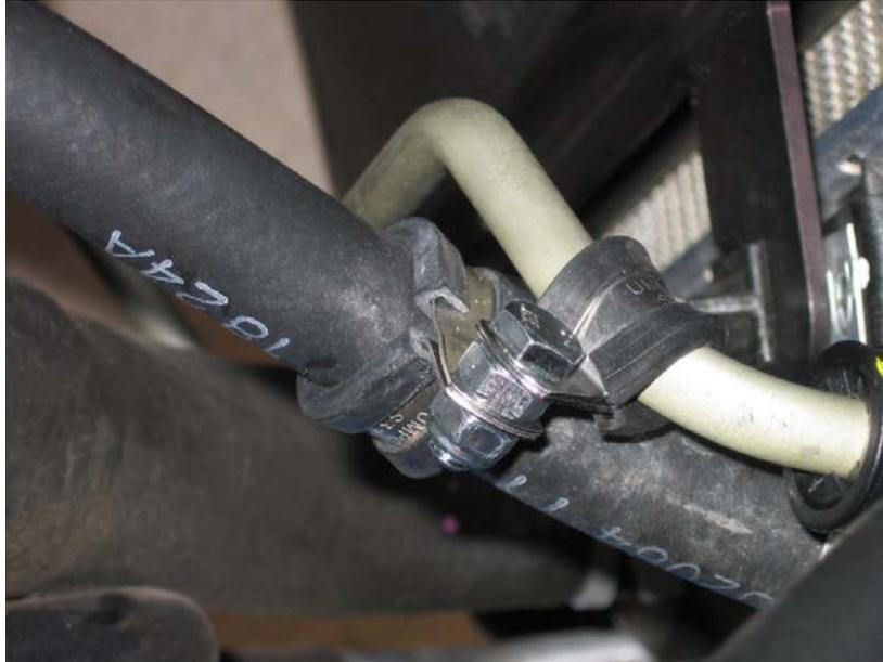
9. Snap the female connector onto the transmission cooler line. Be sure that the clip is fully seated. Slide the black locking cover over the clip. **Note: This photo does not have clip or locking cover shown.**
