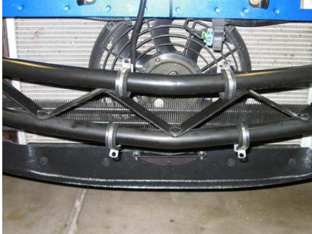
3. Install the cooler. Attach all four mounting points and center the cooler before tightening the clamps. I find it best to hold the bolt and tighten the nut, as the clamps will deform if they rotate with the bolt.
