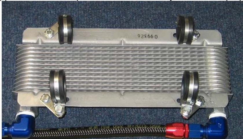
2. Transfer the 4 clamps from the cooler to the crash bars. Note that the orientation of the clamps is maintained. **DO NOT remove the brackets from the cooler.**
