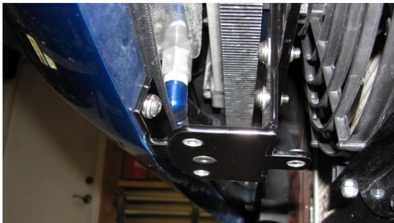
You should now have the forward facing “foot” of the frame mount directly below the fascia mount. Install the flathead screw and locknut back into their original hole. You will need to loosen the two screws that set the vertical height of the “foot” and also position the entire frame mount (left to right) so that everything lines up
