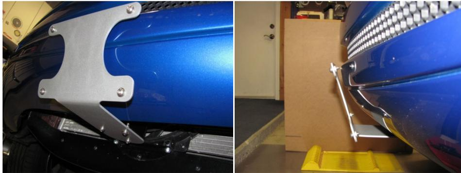
Install your license plate to the aluminum plate holder with the 4 included screws and lock washers.
