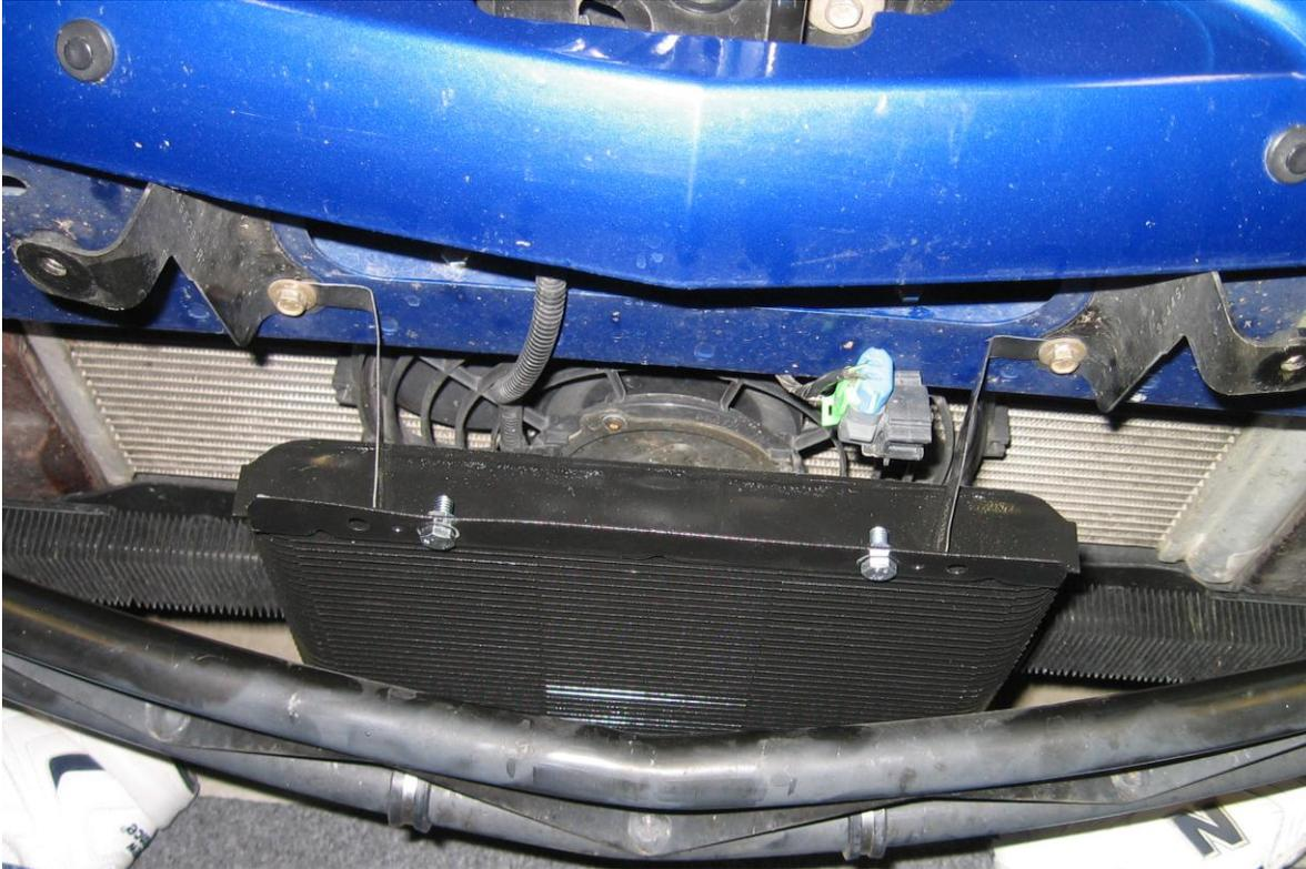
4. Transfer the in-line clamp to the passenger side of the lower crash bar. You will find the clamp has a lock nut separating the two clamps. Leave this in place.
