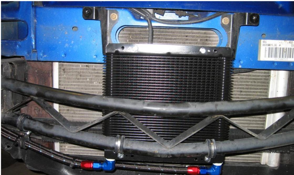
2. Transfer the 2 clamps from the cooler to the lower crash bar. Note that the orientation of the clamps is maintained. **DO NOT remove the upper brackets from the cooler.**
