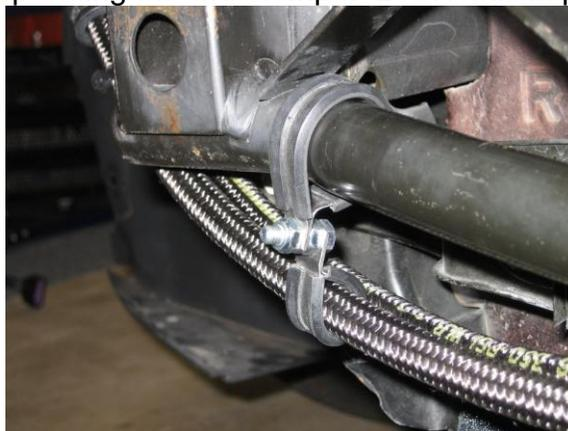
5. Install the twisted bracket to the forward frame-to-body mount point. The bracket goes on the forward side of the mount with the bolt protruding aft. The lines should now be into the engine compartment through the large opening.
