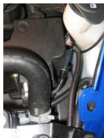
13. Mate the 2 pin fan connector to the wire harness and add tie wraps to hold fan wiring as shown. The center one is horizontally around the vertical part of the hood latch bracket.
