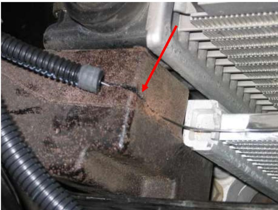
8. Re-install upper radiator mounting panel with the eight bolts removed in step 11. Be sure that the outer bolts do not pinch the corrugated tubing passing under them. You now have the temperature probe installation complete. Re-install the air box assembly onto the upper radiator mount panel.
