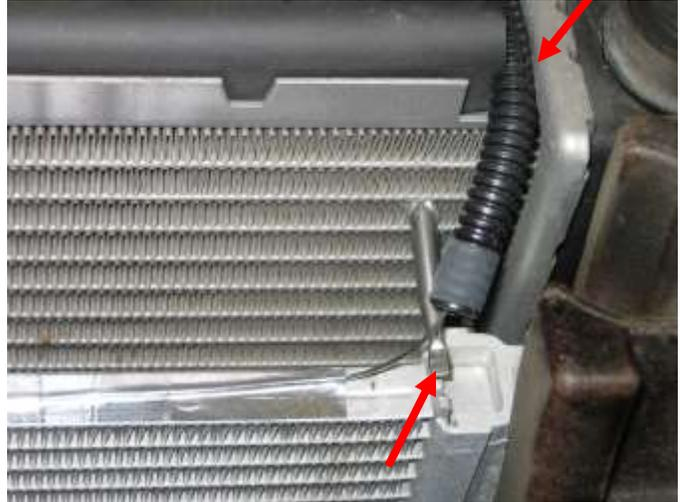
7. Put a small slice in the pad on the passenger side of the radiator, so that the capillary tube is aligned with the A/C condenser. This is also a good time to burnish down the aluminum tape so that it is a permanent installation. You won't be seeing this spot again for a long time.
