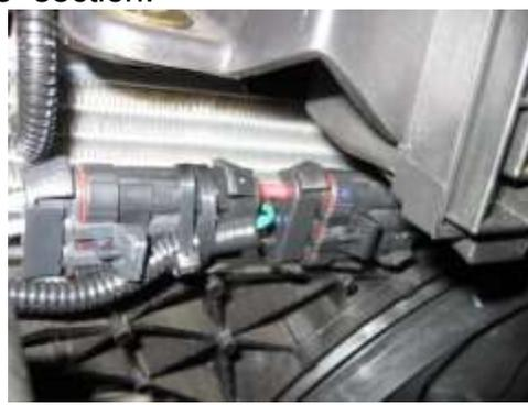
12. Mate the single pin connector (with the green wire) to the harness and stow the fuse holder along fender.
