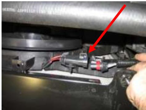
10. Remove engine compartment fuse block outer cover.
