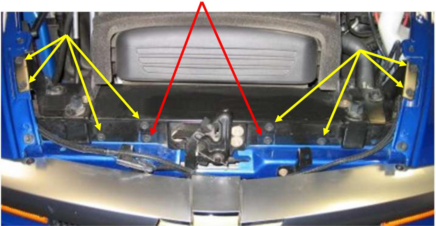
12. Remove right forward fender mounting bolt.
