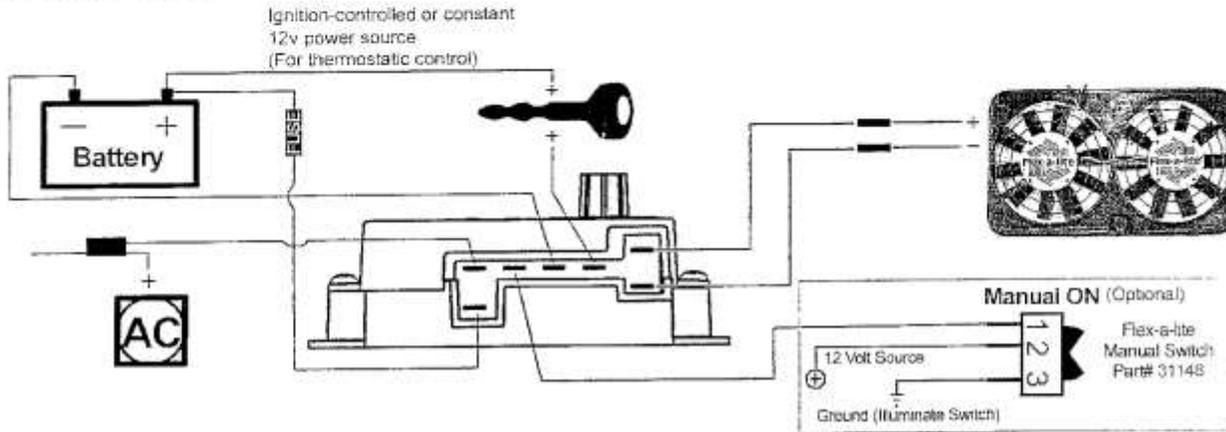
**Step 2:** Wire the fan motor (s) (refer to above wiring diagram. Connect the fan motor wires to the control module (positive wire to the "M+" terminal and negative motor wire to the "M-" terminal). **Note:** Be sure to use wire that is intended to handle the current (amp) rating of the fan.
