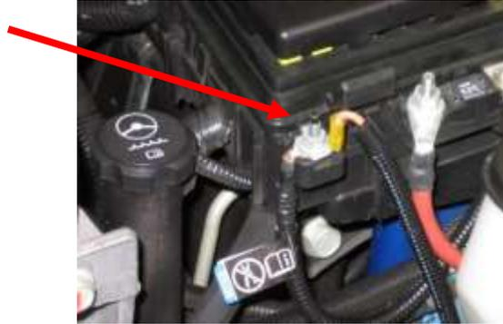
10. Re-install the fuse block outer cover. Be careful to route the new wire to clear the cover.
