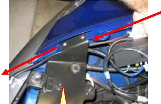
Note: Upper radiator mount shown installed for routing reference only.
