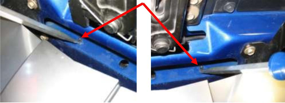
7. After dropping the wire harness from the cross-frame, remove the two wire harness clamps from the harness. You will be installing one of them in the center of the upper fan bracket.
