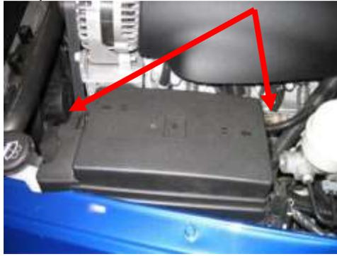
11. Remove 8 (the two sets of four) mounting bolts on the upper radiator mounting panel in order to remove the panel assembly from the truck. **DO NOT** remove the two that hold the hood latch to the cross member, or you may mess up your hood adjustment!!! They are the **BOTTOM** two of the hood latch attachment. The hood latch will remain connected to the cross member.
