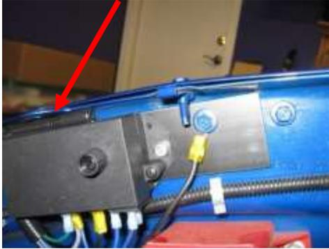
2. Route the controller wiring harness forward along the fender so that it will pass under the (currently removed) radiator mounting panel. There will be enough room for everything when re-installing the panel.
