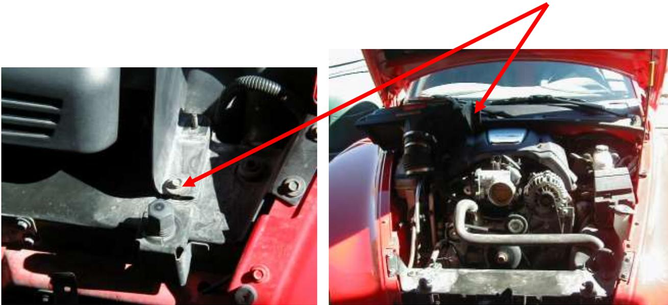
5. Remove cross member air guide with a flat tip screw driver to push down and pry away from the cross member, and pull forward and out to expose the wiring harness mounts.
