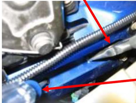
4. While holding the upper mount bolts, loosely install both nylon locking nuts. If you have an '06, your temp sensor is on a metal bracket attached to the left wiring harness mount, you can relocate the bracket under the nut of the left mount bolt. This is difficult to do and requires extra hands. Earlier models may have the temp sensor taped to the wire harness. You can either leave this as is, or tie wrap the sensor to the harness.
