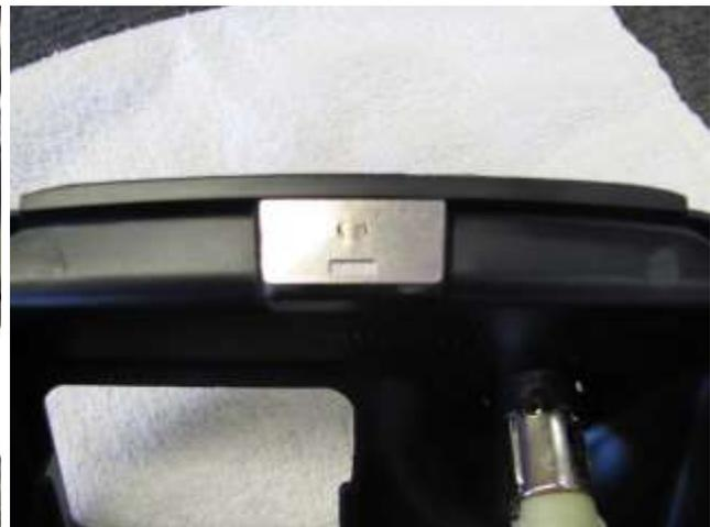
5. Mix up a little of your favorite epoxy, apply it and clamp the part in place. I found a pair of clothes pins worked great. Be certain that the repair part is exactly centered, left-to-right and that the metal is firmly against the outer edge of the plastic part.
