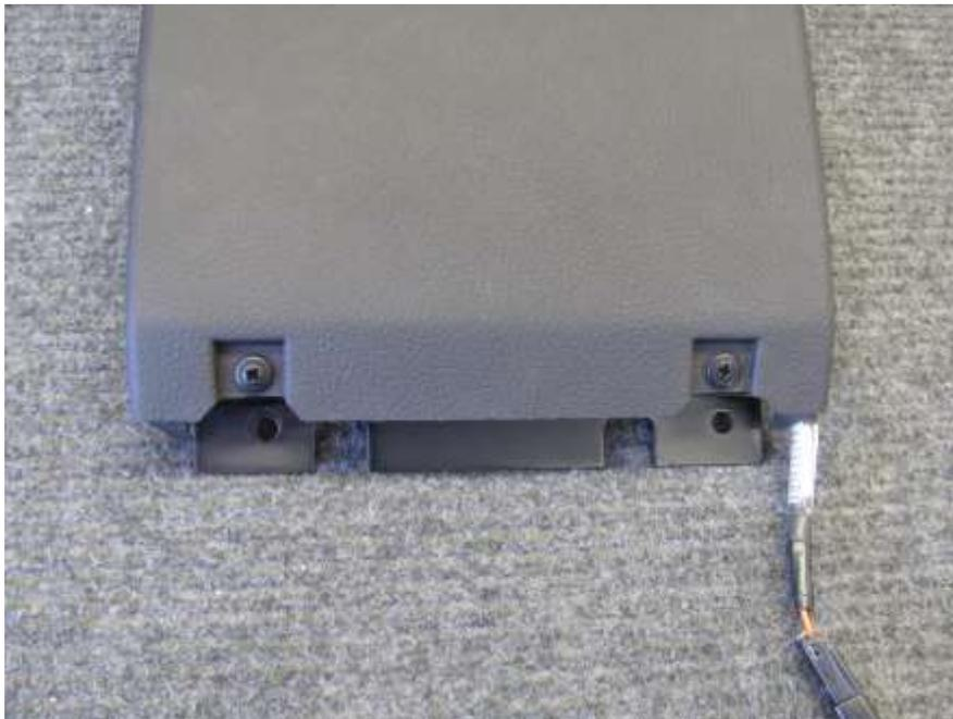
2. Here is what your broken part looks like on the bench. Have a careful look at the receiver part of the latch in the dash and be sure the broken post is not still lodged in there. You can also carefully “test” the new metal part into the dash latch to verify operation. Proper alignment of the post into the receiver is critical, so be patient..... You should be able to latch and unlatch the metal post by itself.
